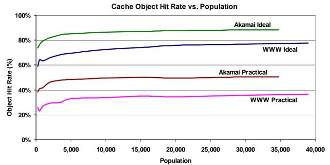
**Figure 13. WWW and Akamai object hit rates vs. population:** object hit rates as a function of population size. An ideal cache treats all documents as cacheable. A practical cache accounts for HTTP 1.1 caching directives. All simulations used an infinite-capacity proxy cache.
