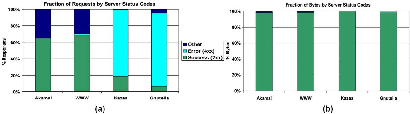
**Figure 12. Server status codes:** response codes returned by external servers; (a) shows the fraction of requests broken down by response code, (b) shows the fraction of bytes broken down by response code.
