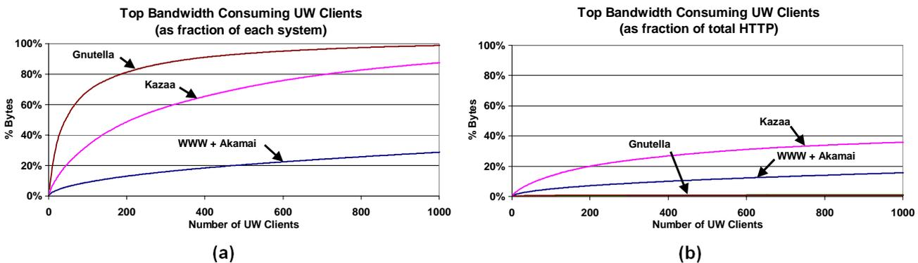
**Figure 7. Top UW bandwidth consuming clients:** a CDF of bytes downloaded by the top 1000 bandwidth-consuming UW clients (a) as a fraction of each system, and (b) as a fraction of the total HTTP traffic.
